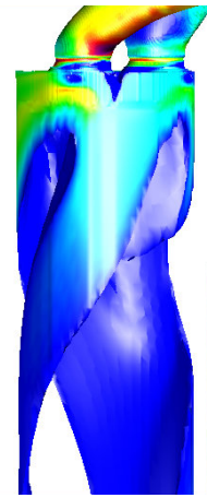
Figure 2: The swirling motion of flow in the combustion chamber of a diesel engine (side view) as illustrated by an isosurface. This is a velocity isosurface with an isovalue of 5.0 m/s. Any CFD attribute can be mapped to hue.
