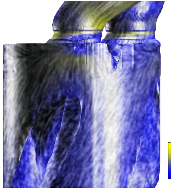
Figure 6: (color plate) A close-up of a velocity isosurface from Figure 3: with texture-based flow visualization and a normal mask applied. With the texture advection on the isosurface, it is clear that the ideal swirl flow pattern is not exhibited in this region.
