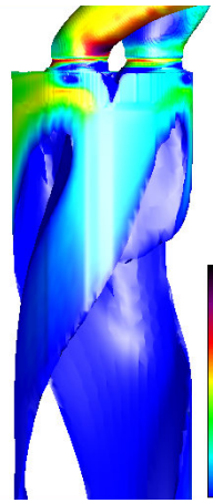
Figure 5.2: The swirling motion of flow in the combustion chamber of a diesel engine (side view) as illustrated by an isosurface of velocity. This is a velocity isosurface with an isovalue of 5.0 m/s. Any CFD attribute can be mapped to hue.
