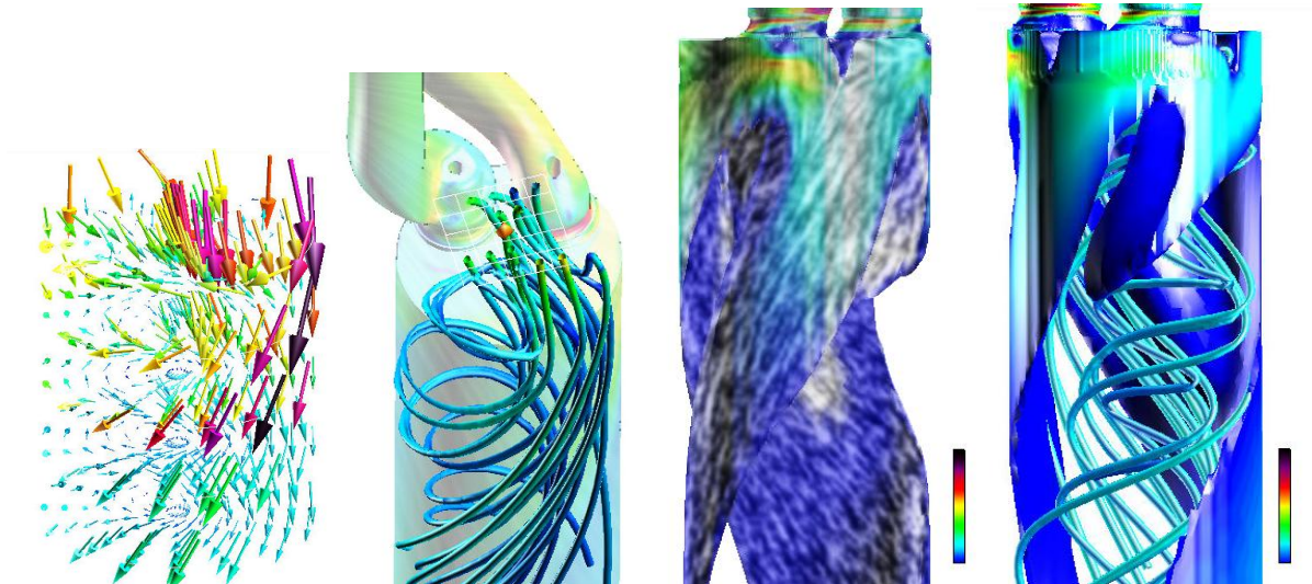
Figure 7.6: The visualization of swirl flow in the volume of the the combustion chamber: (left) direct visualization using color-mapped glyphs, (middle-left) geometric flow visualization using color-mapped shaded streamlines, (middle-right) texture-based flow visualization on a velocity isosurface, and (right) isosurfacing combined with 3D streamlines.
