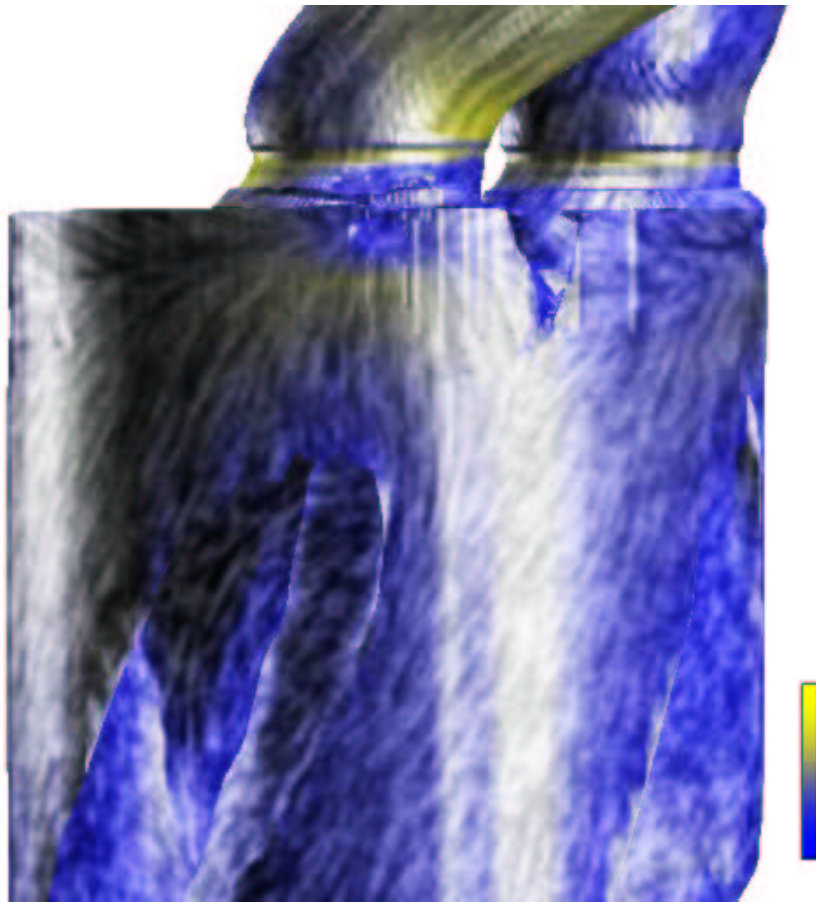
Figure 5.8: A close-up of a velocity isosurface from Figure 5.5: with texture-based flow visualization and a normal mask applied. With the texture advection on the isosurface, it is clear that the ideal swirl flow pattern is not exhibited in this region.
